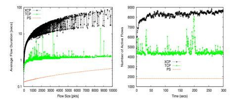
Fig. 1. The plot on left shows the average flow duration versus flow size under TCP and XCP from a simulation with Poisson flow arrivals, flow sizes are pareto distributed with mean = 30 pkts (1000 byte/pkt) and shape = 1.4, link-capacity = 2.4 Gbps, RTT = 100 ms, offered load = 0.9. The plot on right shows the the number of active flows versus time. In both plots the PS values are computed from analytical expressions
