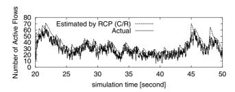
Fig. 3. Comparison of the number of measured active flows and the estimate (C/R). Bottleneck capacity, C = 10Mb/s, RTT = 50ms, flow arrival rate = 400 flows/sec, and flow sizes are pareto with mean = 25 pkts (1000 byte/pkt) and shape parameter is 1.2
