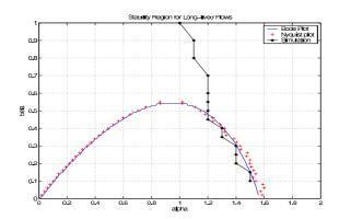
**Fig. 4.** Region enclosed by the solid curve is the stability region obtained via Bode and Nyquist analysis. The region to the left of the '-\*' line is the stability region of the non-linear system obtained from simulations and phase plane method
