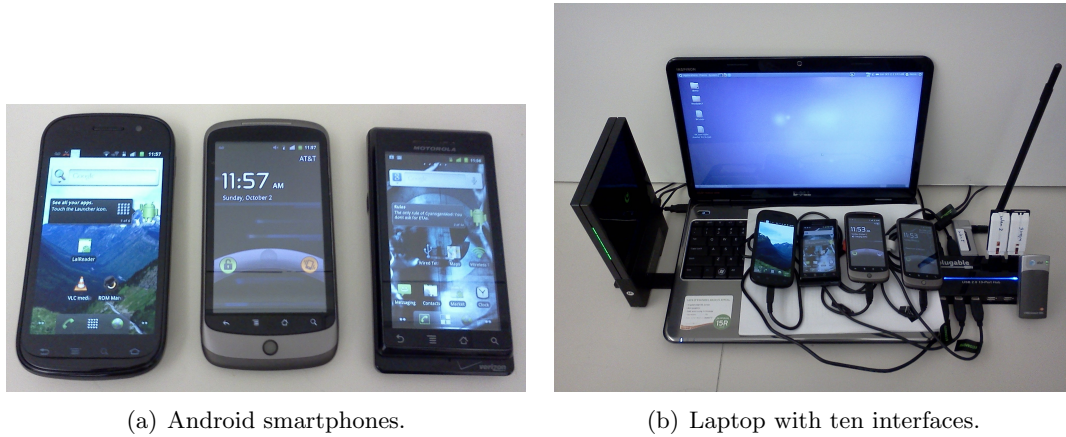
Figure 2.2: Devices on which the Hercules network stack is run, allowing them to exploit multiple networks at the same time.
