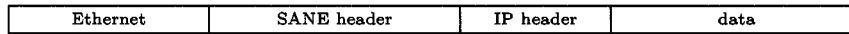
Figure 2.3: SANE operates at the same layer as VLAN. All packets on the network must carry a SANE header at the isolation layer , which strictly defines the path that packet is allowed to take.
