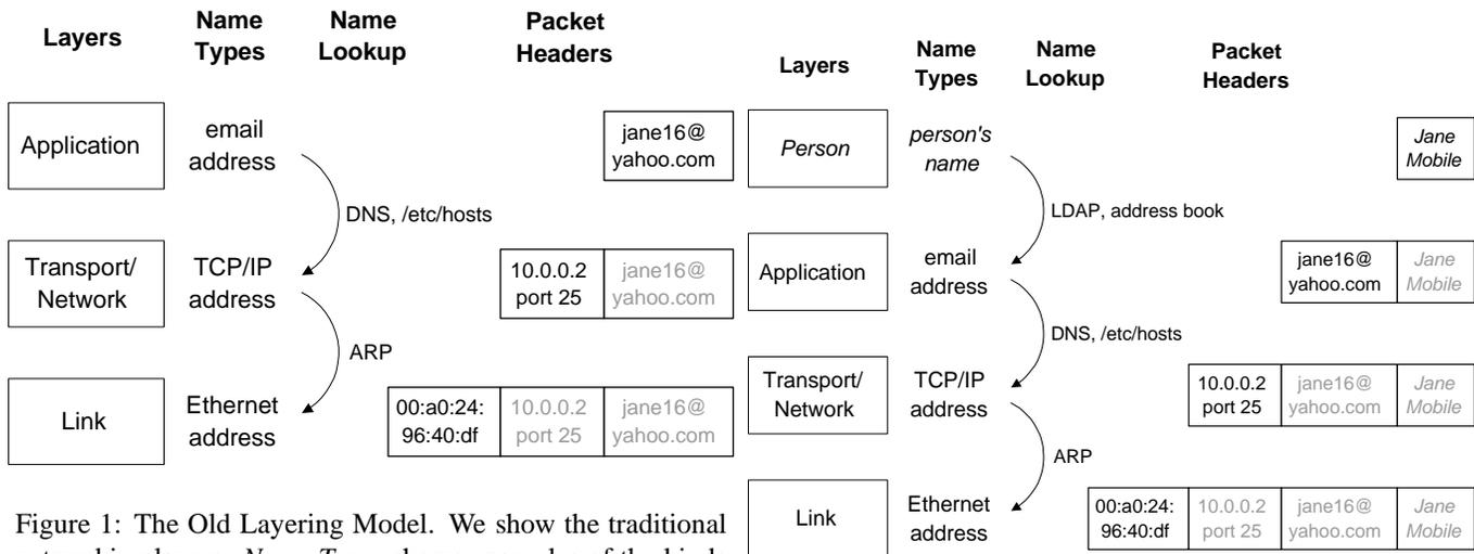
Figure 1: The Old Layering Model. We show the traditional networking layers. *Name Types* shows examples of the kinds of names used at each layer. *Name Lookup* shows some methods of mapping names from each layer to names in the next lower layer. *Packet Headers* shows examples of actual names at each layer, and their relative locations in a typical email packet.
