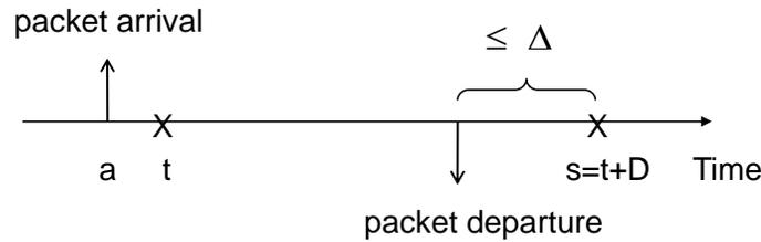
Figure 5.3: Packet scheduling under BJP. A packet that arrives at time  $a$  is scheduled based on its arrival time stamp  $t \geq a$ . The packet is scheduled to depart the buffer as close to  $t + D$  as possible, where  $D$  is a constant delay.
