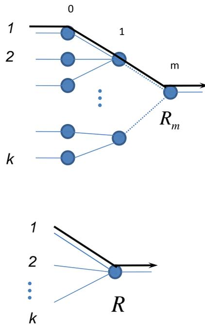
Figure 5.1: Tree-structured network (top). The buffer occupancy of router  $R_m$  in this network does not exceed the buffer occupancy of an isolated router  $R$  into which the ingress traffic is directly fed (bottom).
