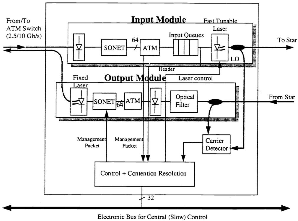
Fig. 3. Proposed interconnection node: Input + Output Modules
