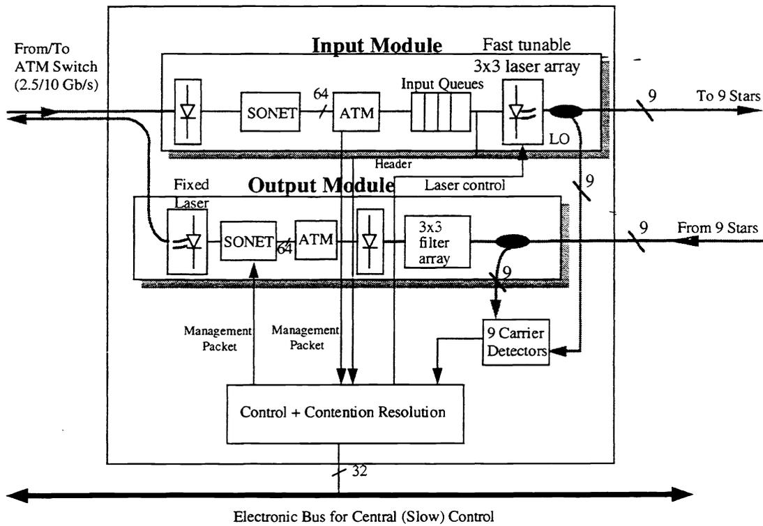
Fig.12. Proposed interconnection node utilizing a 3x3 optical subnetworks scheme
