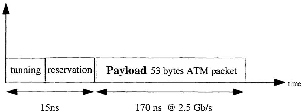
Fig. 5. Optical transmission time slots
