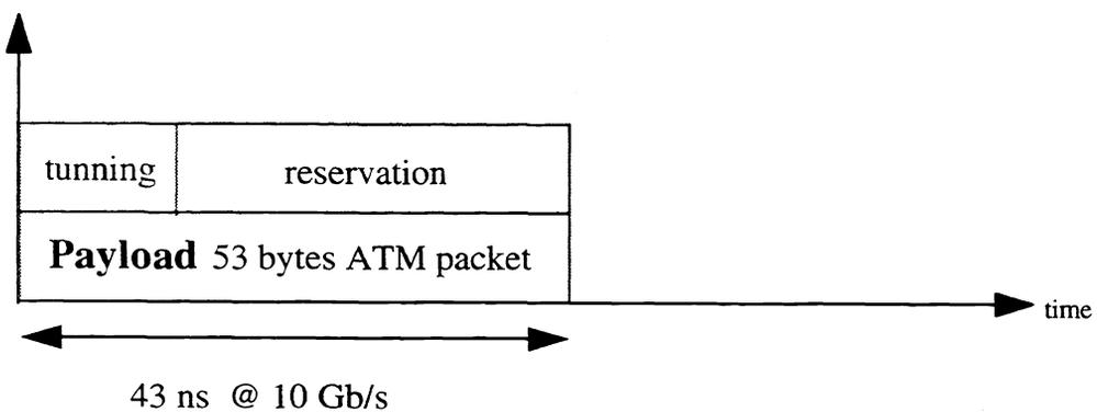
Fig. 7. Optical transmission time slots for a system with parallel payload and reservation channels.
