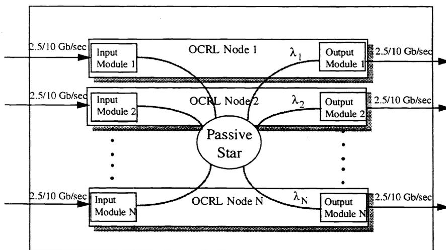
Fig. 2. Proposed interconnection multi Tb/s ATM/WDM site (a single rack)
