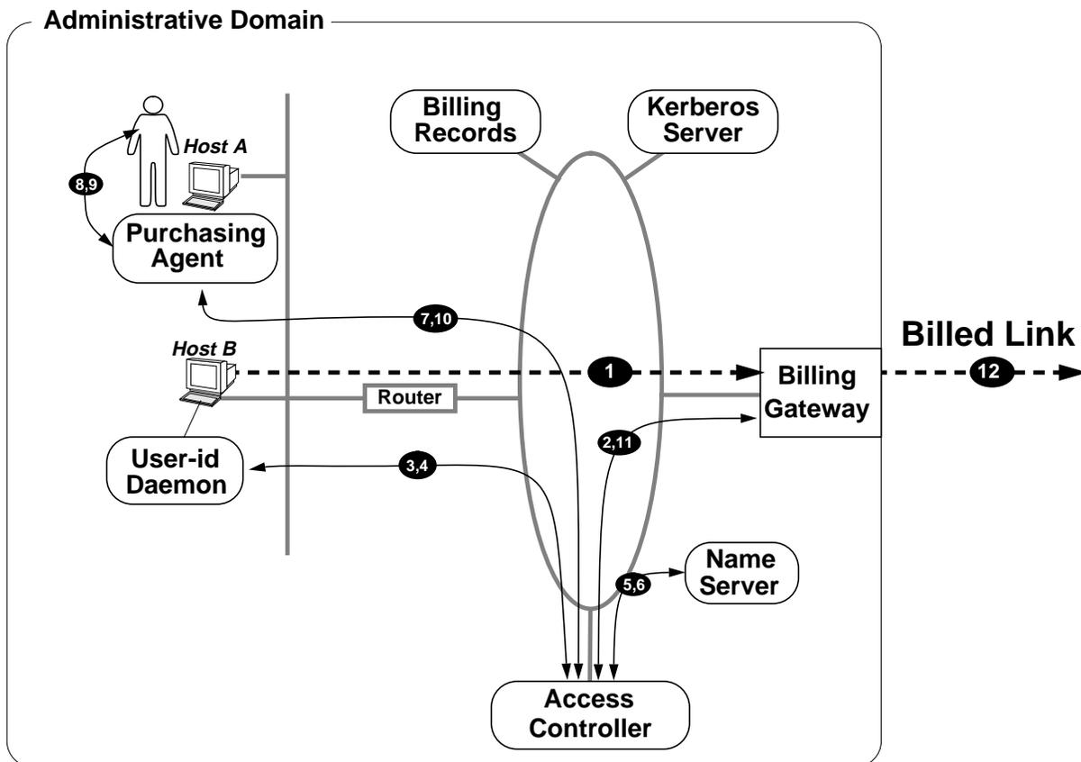
**FIGURE 1.** Components of the billing systems showing the major communications required to establish a connection.
