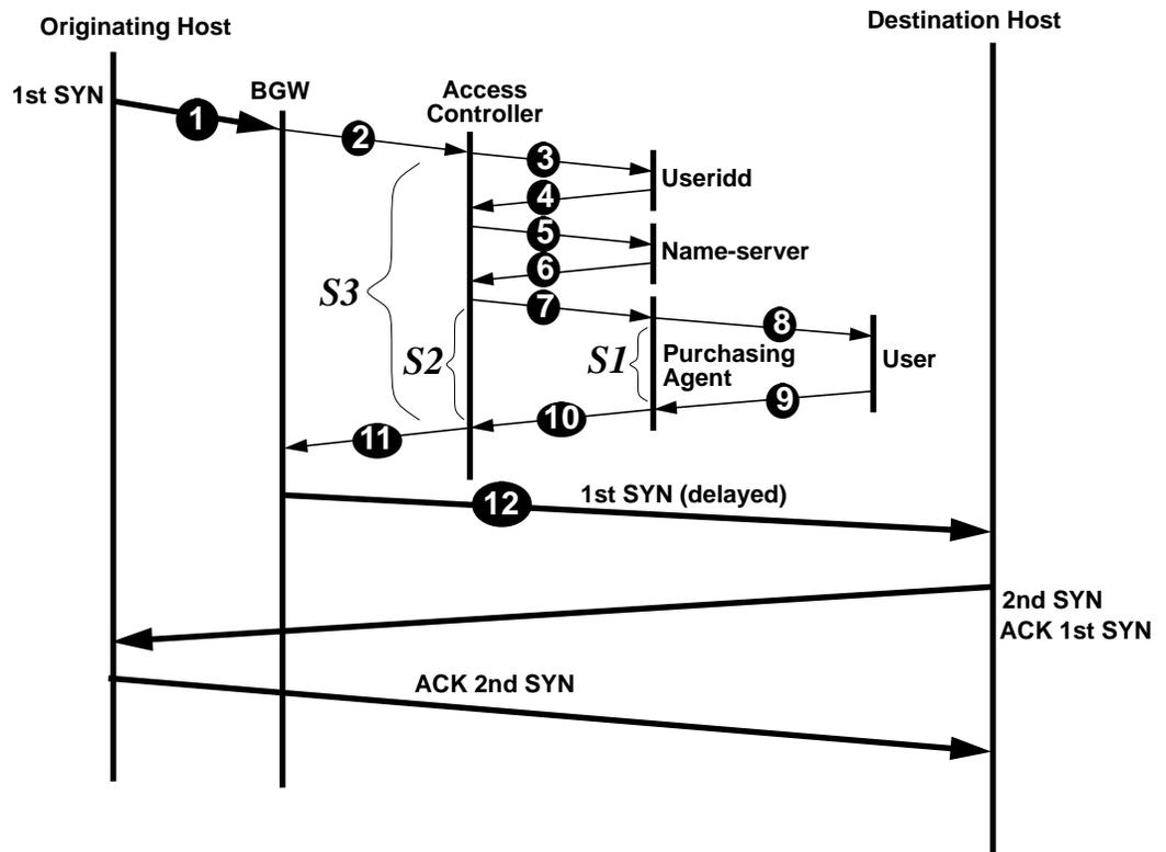
(b) Billing System Communications Involved in Establishing a Connection
