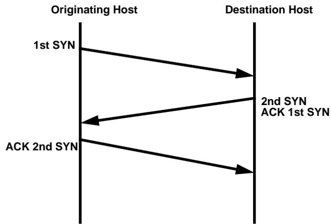
(a) Normal 3-Way handshake to establish connections
