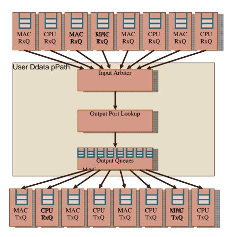
Fig. 5: NetFPGA's Router Data Path
