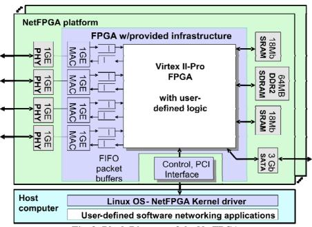
Fig. 3: Block Diagram of the NetFPGA
