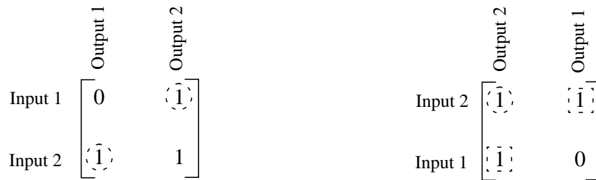
a) Original request matrix with a WFA match shown by the circles.
