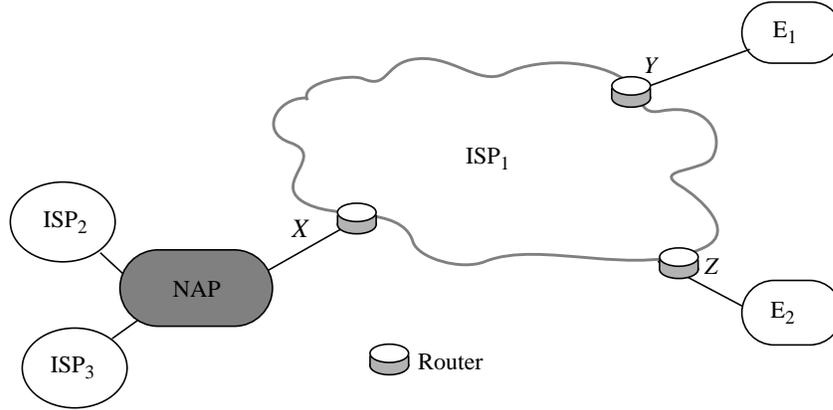
**Figure 2** Example network of an ISP (ISP<sub>1</sub>) connected to two enterprise networks (E<sub>1</sub> and E<sub>2</sub>) and to two other ISP networks across a network access point (NAP).
