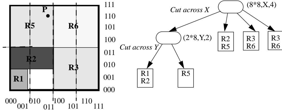
**Figure 15** A possible HiCuts tree for the example classifier in Table 5. Each ellipse in the tree denotes an internal node  $v$  with a tuple (size of 2-dimensional space represented, dimension to cut across, number of children). Each square is a leaf node which contains the actual classifier rules.
