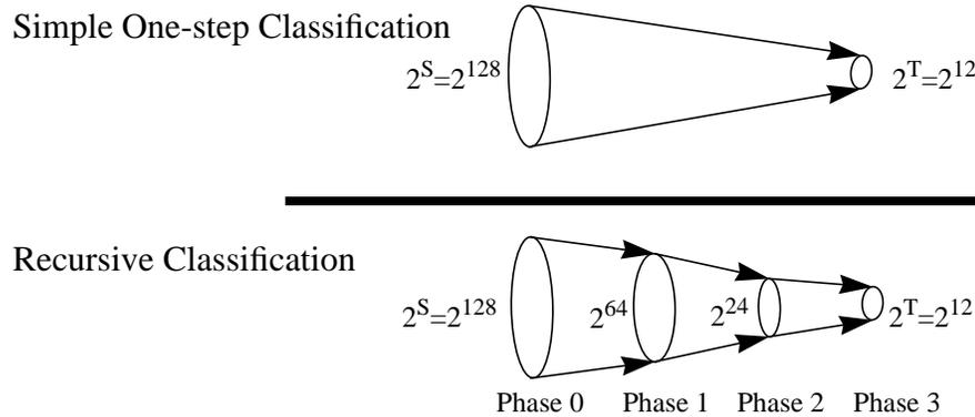
**Figure 13** Showing the basic idea of Recursive Flow Classification. The reduction is carried out in multiple phases, with a reduction in phase  $I$  being carried out recursively on the image of the phase  $I-1$ . The example shows the mapping of  $2^S$  bits to  $2^T$  bits in 3 phases.
