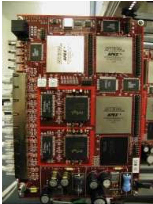
Figure 1: NetFPGA Board: an 8 port, programmable network device
