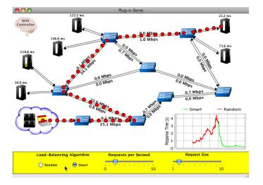
Figure 1: The frontend GUI shows the up-to-date state of the system and allows the user to control various parameters. The state of each server can be toggled by clicking. OpenFlow channels requests to different servers, or through different paths to the same server.
